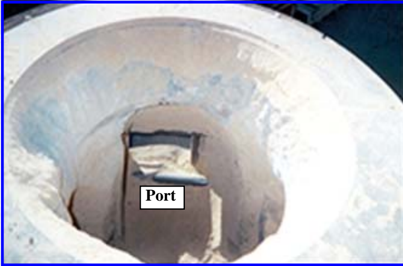
Rock-Packed Rotor/Balancer Assembly Port Holes are protected on three sides with tungsten carbide wear parts.
