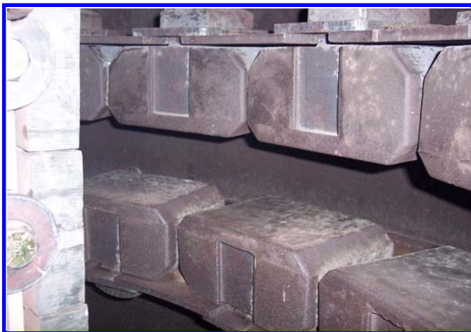
Anvils in top and bottom rock shelves insure solid rock pack. Anvils last 3000 to 5000 hours. Anvils in top can be rotated 180 degrees and used in the bottom because of the wear pattern.
