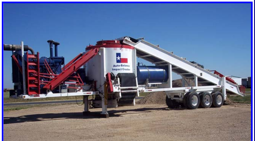
Hydraulic System on Legs raises Crusher so Trailer can back under the Crusher. Eliminates need for Crane to load or unload the Crusher. Portable without expense of a chassis.
