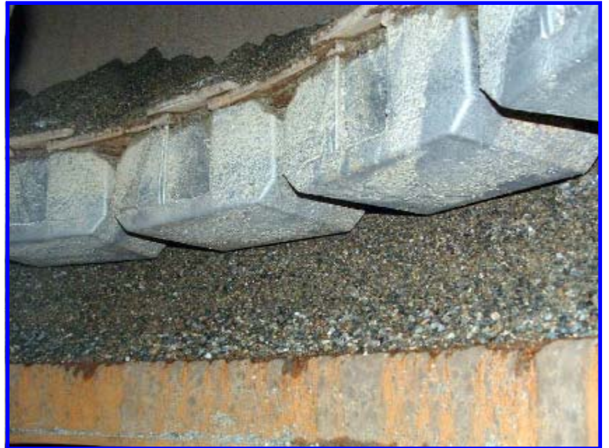
Rock-Packed Crushing Chamber Anvils used in the top rock shelf and vertical flange in the bottom rock shelf insure a solid material pack
