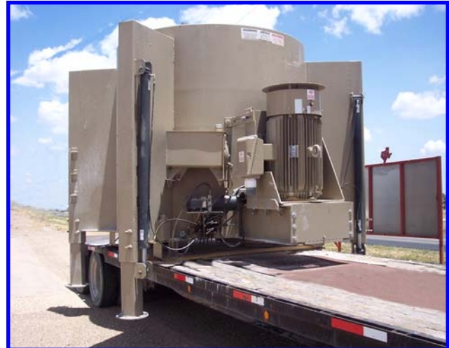
Hydraulic System on Legs raises Crusher so Trailer can back under the Crusher. Eliminates need for Crane to load or unload the Crusher. Portable without expense of a chassis.
