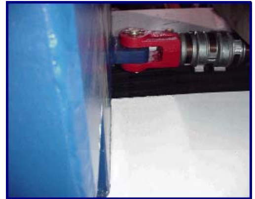
Hydraulic Cylinder attaches to Motor Stand and to Pump
