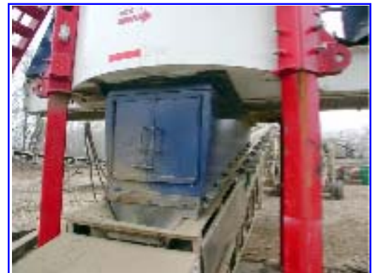
Crusher to Conveyor Discharge Box: 16 degree angle with Door for entrance through bottom of Crusher for inspection and mainte- nance. Properly enclosed, helps to minimize dust escaping from Crusher.
